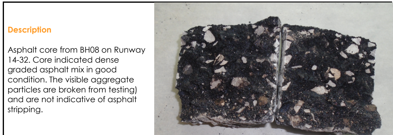
Figure 7 Asphalt Core from Runway 14-32
