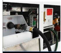
AEROPAL LT fueling hoses are optimized for an operating temperature range of -48 ° C to +70 ° C.
