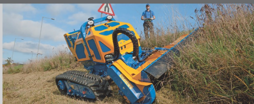
Bomford Flailbot Remote Controlled Steep Slope Mowers
