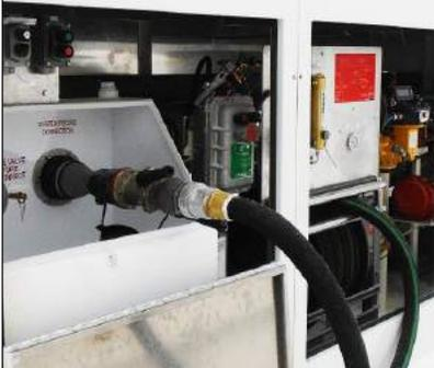
**AEROPAL LT** fueling hoses are optimized for an operating temperature range of  $-48^{\circ}\text{C}$  to  $+70^{\circ}\text{C}$ .
